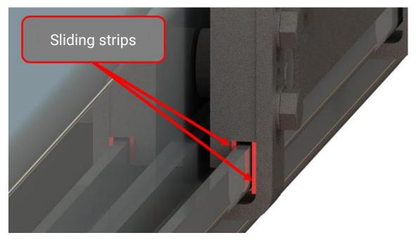
• Cut the sliding strips (art. no. 23003131) to size and affix them to the side part and the withdrawal protection device.
