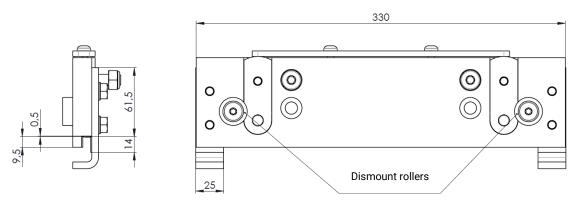
• Then dismount the rollers which were previously used for guiding the axle jack.
