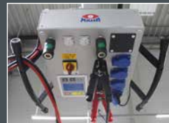
Lift control, power supply, compressed air and data socket positioned on bottom side.
