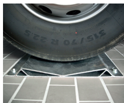
Wheel recesses serve as positioning assistance for vehicle lifting. They are either fixed or movable.
