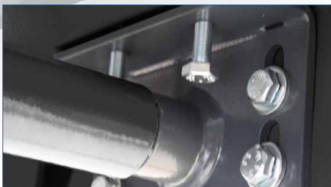
Adjustable bearing enables independent alignment of runway to scissors.
